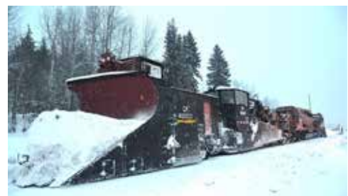
CP Plow/Spreader Consist Heavy duty snow plow and sand spreading operations.
