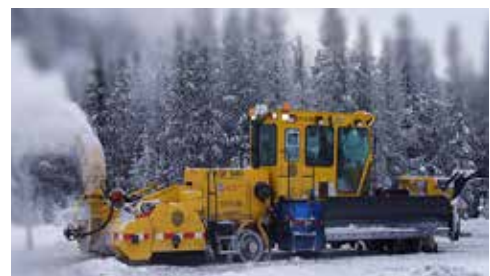
CP Snowfighter Smaller multi-purpose snow clearing equipment plows, spreads sand and blows snow.
